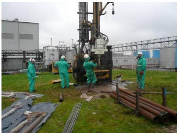
Fig 2 Sonic core sampling on contaminated site
